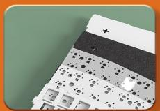
Filled with 5 Layer Silent Material, effectively reduce gap among switches and typing noise
